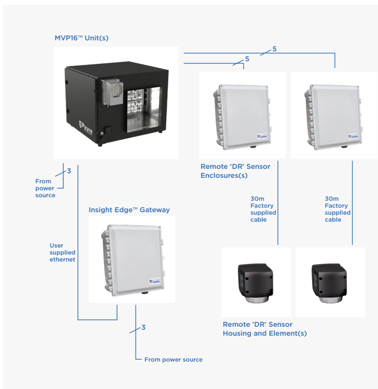
Figure 4: MVP16 System sample configuration with two Remote 'DR' Sensors
